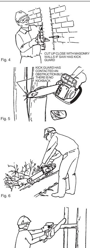
4. When cutting piled up brush, don't stick the saw blade into the pile unless it has a Kick Guard. (See Fig. 6.)
